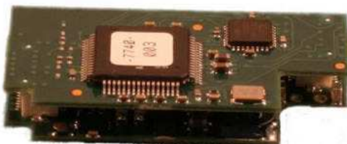
(TS//SI//REL) FLUXBABBITT Hardware Implant for PowerEdge 2950
